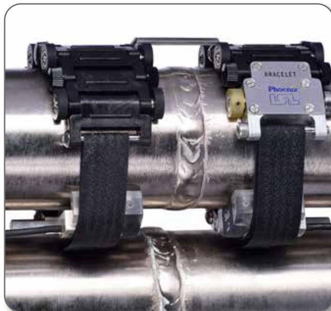
Dual Bracelet configuration scanning double sided phased array on 2" pipe
